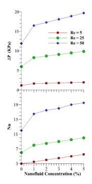
Fig. 3. Nu and pressure drop at lower Re and nanofluid concentrations.
