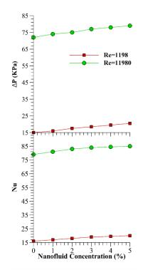
Fig. 4. Nu and pressure drop at higher Re and nanofluid concentrations.
