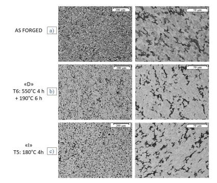
Fig.2 - Microstructure of as forged condition (a), "D" T6 heat treatment (b) and "I" heat treatment (c).
