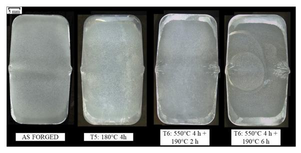
Fig.1 - Grain structure across section of samples in the as forged and heat-treated conditions.
