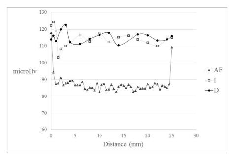
Fig.3 - Microhardness profile of As Forged (AF) condition, "D" T6 heat treatment and "I" heat treatment.
