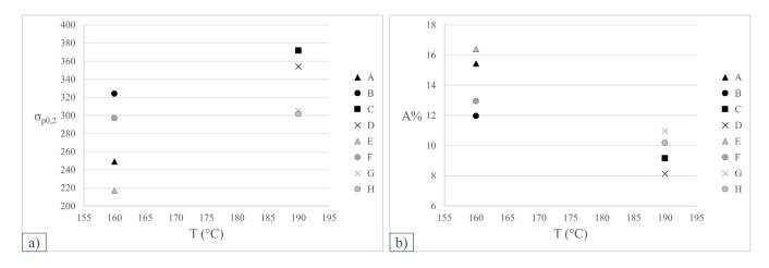
Fig.4 - Effect of temperature on yield strength and elongation of EN AW6082 T6 Al alloy.
