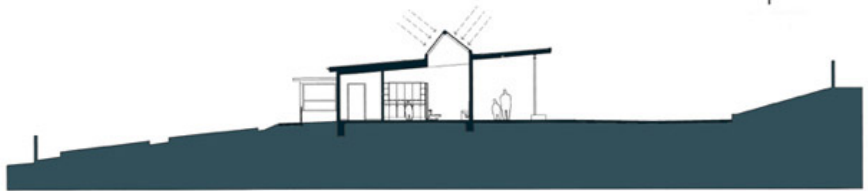
Section through skylight- PV cells on south face, skylight from north face
