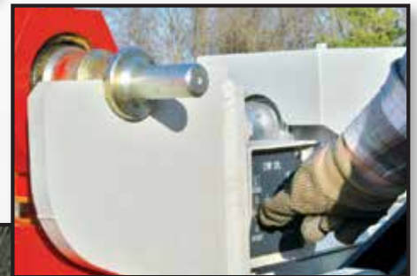
Counterweight removal control station
