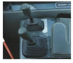
Kick-down switch is conveniently located on the mono-lever. A simple motion of the thumb actuates this valuable productivity feature.
