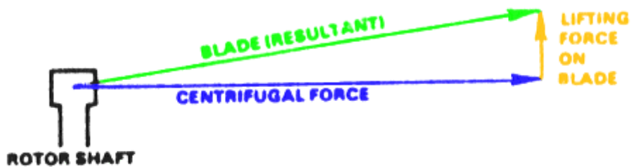
FIGURE 2-33. RESULTANT OF LIFT AND CENTRIFUGAL FORCES.
