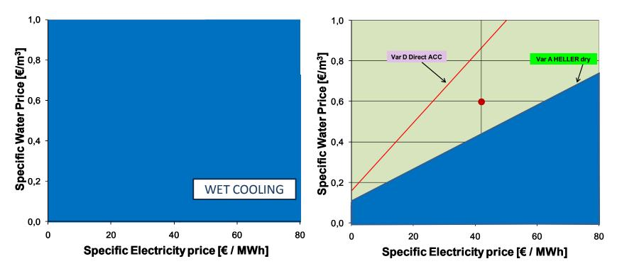
The all-dry HELLER System (var. A) is competitive against wet cooling (var. E) - at an assumed water price of 0.6 €/m<sup>3</sup> – up to 63.5 €/MWh electricity selling price.
