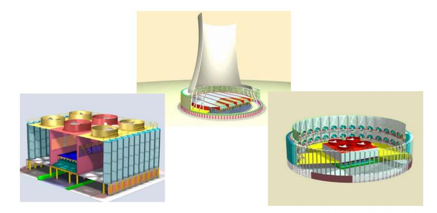
Conceptual designs for wet assisted HELLER Systems locating the assisting cells in the main dry cooling tower
