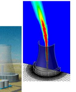
• A single tower shell serves two 160 MW<sub>e</sub> power units
