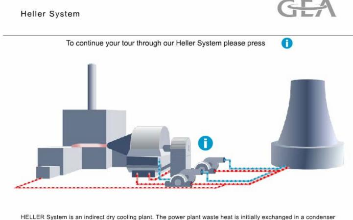
HELLER System is an indirect dry cooling plant. The power plant waste heat is initially exchanged in a condenser (preferably a direct contact one) to a closed cooling water circuit. The heat absorbed by the water is rejected to ambient air in fin tube type heat exchangers. Air moving can be either by natural or mechanical draft. © GEA Energy Technology GmbH
