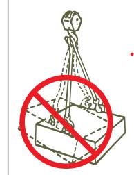
Do not shock load. Jerking the load could overload the sling and cause it to fail.
