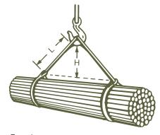
Vertical Choker rating of each sling = 6,000 lbs. Measured Length (L) = 6 ft. Measured Height (H) = 4 ft. Reduction Factor (RF) =  $4 (H) \div 6 (L) = .667$ Reduced sling rating in this configuration = .667 (RF) x 6,000 lbs. = 4,000 lbs. of lifting capacity per sling
