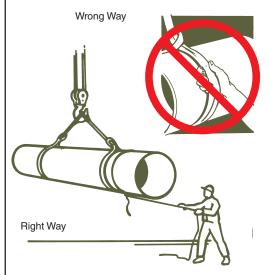
After lifting, the load should not be pushed or guided by employees hands directly on the load. Ropes or "tag lines" should be attached for this purpose.
