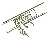
Rated capacities (Working Load Limits) must be shown by markings or tags attached to all slings.
