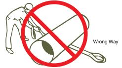
Before a load is lifted, a place should be prepared where it is to be put down. Lumber can be used to allow space to remove the sling and prevent shifting of the load.
