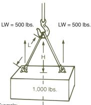
Example: Load weight = 1,000 lbs. Rigging - 2 slings in vertical hitch Lifting Weight (LW) per sling = 500 lbs. Measured Length (L) = 10 ft. Measured Height (H) = 5 ft. Tension Factor (TF) = 10 (L)  $\div$  5 (H) = 2.0 Minimum Vertical Rated Capacity required for this lift = 500 (LW) x 2.0 (TF) = 1000 lbs. per sling
