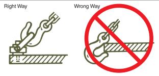
Do not point load hooks - center load in base of hook.
