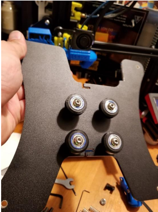
This is eccentric nut (with wheel removed for clarity) in the fully tight position
