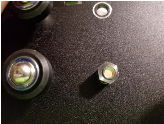
This is the eccentric wheel in the fully loose position where through bolt is furthest away from the fixed idler wheels (left side in photo).
