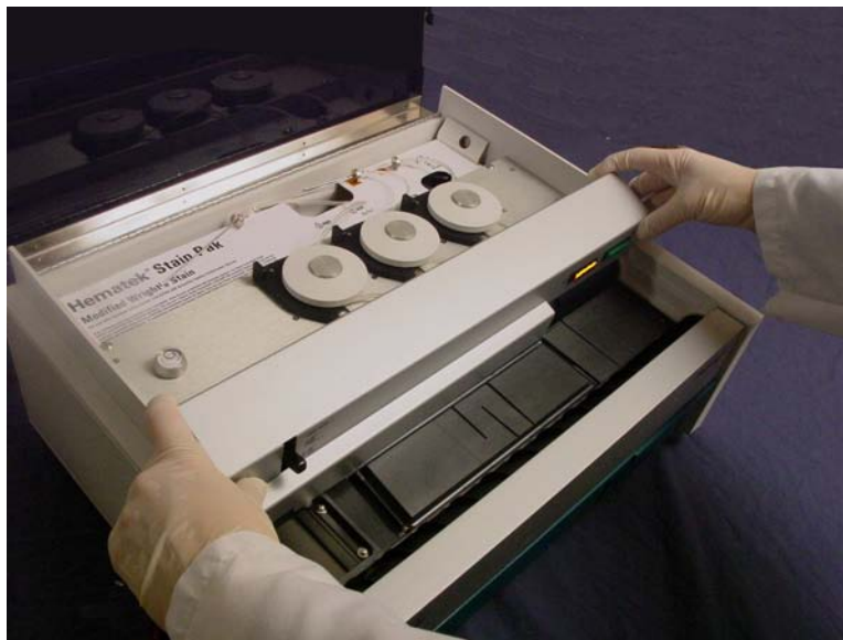
Figure 6-4. Raising the Circuit Board Cover
