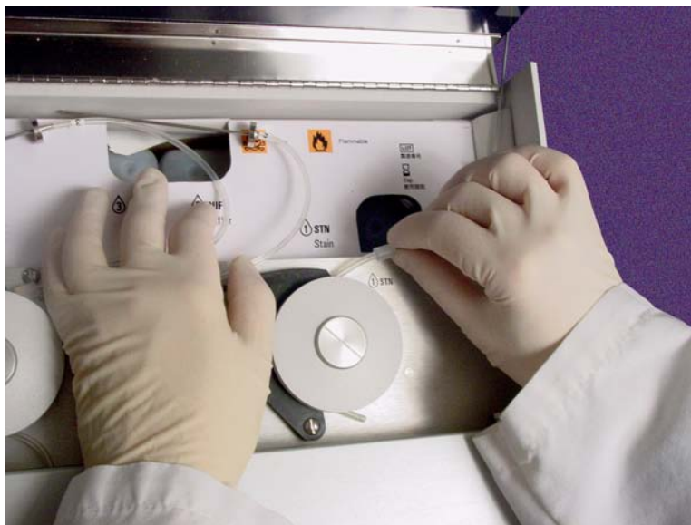
Figure 6-11. Inserting Tubing into Pump Assembly
