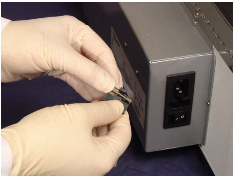
Figure 6-2. Replacing the Fuse
