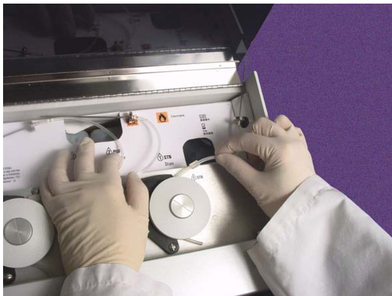
Figure 6-10. Removing Tubing from Pump Assembly
