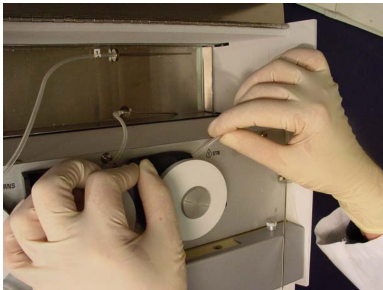
Figure 2-3. Threading Tubing through Pump Assembly
