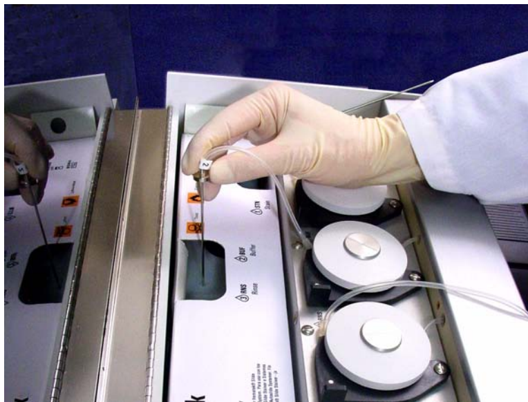
Figure 2-6. Installing Cannula into Stain Pak Bottle
