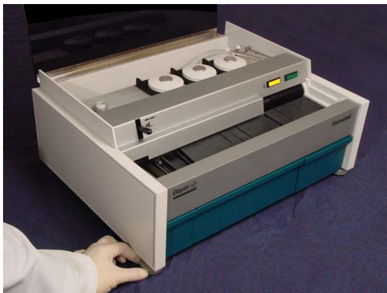
Figure 2-1. Leveling the Instrument
