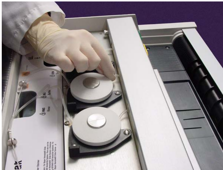
Figure 6-9. Removing Tubing from Nipple
