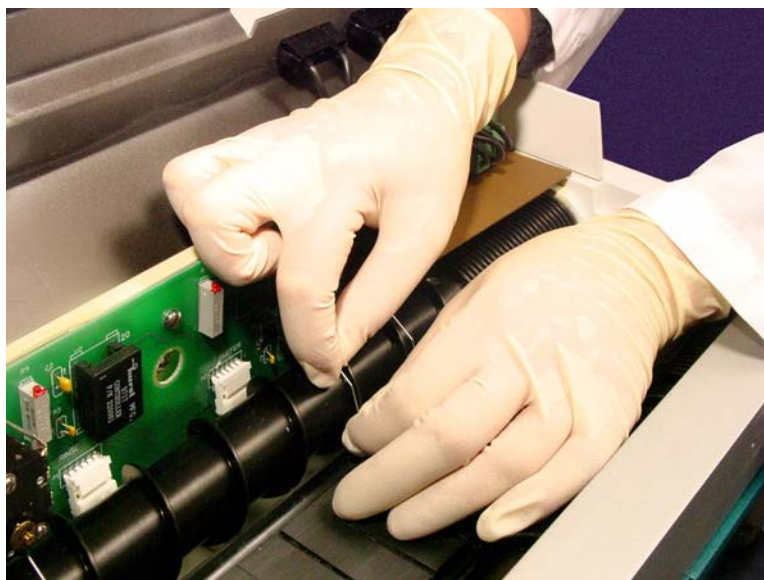
Figure 6-19. Adjusting the Sensing Switch Finger
