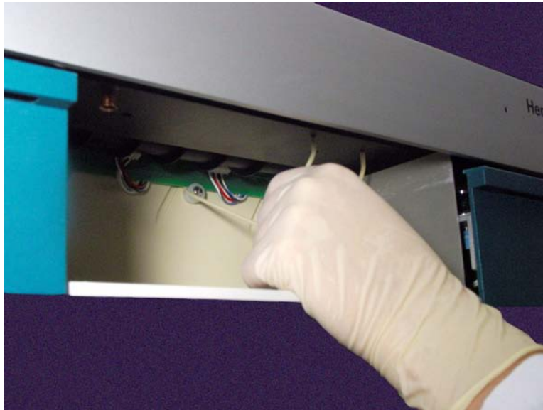
Figure 6-16. Connecting Underplaten Tubing to Platen Spout
