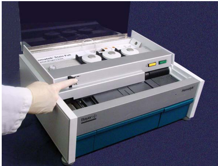
Figure 3-1. Priming the Tubing
