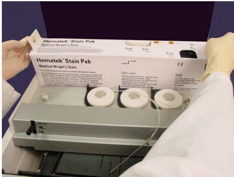
Figure 2-5. Installing the Stain Pak
