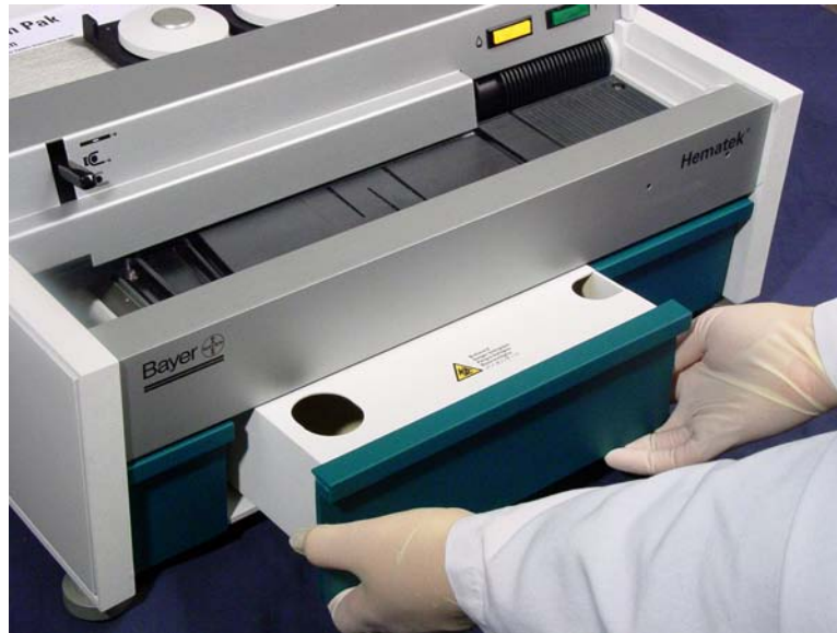
Figure 5-3. Removing the Waste Tank
