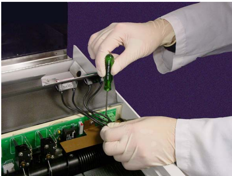
Figure 6-5. Removing the Connector Wires
