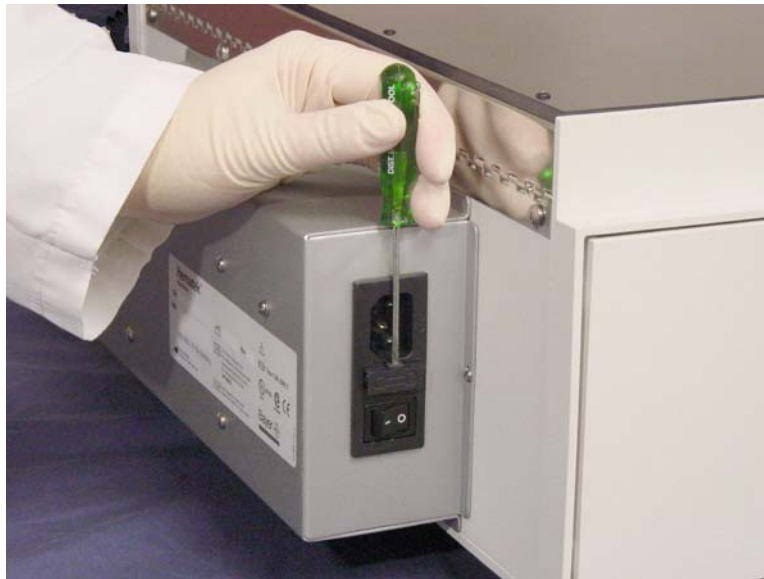
Figure 6-1. Opening the Fuse Cover
