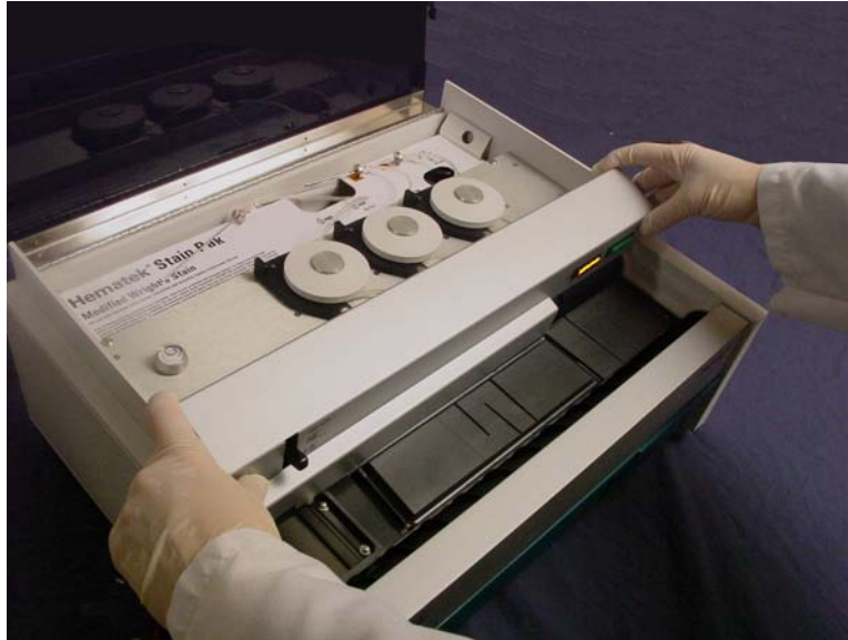
Figure 5-5. Raising the Circuit Board Cover
