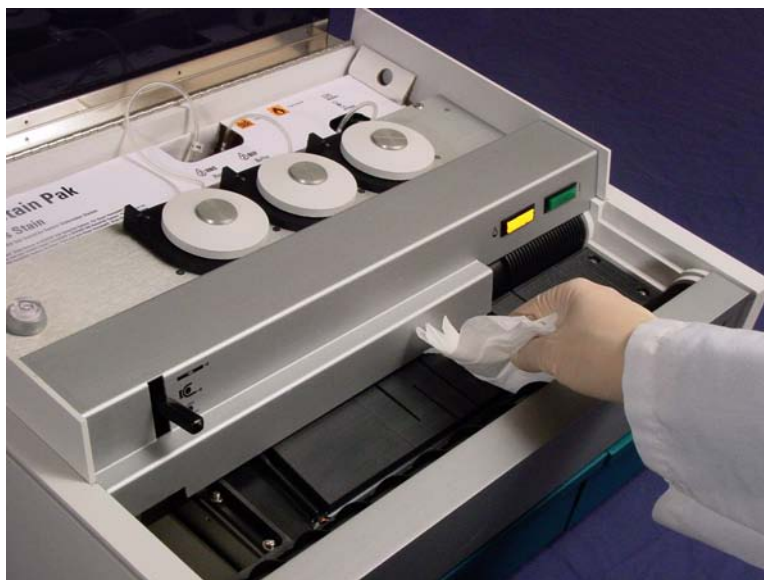
Figure 5-1. Cleaning the Platen
