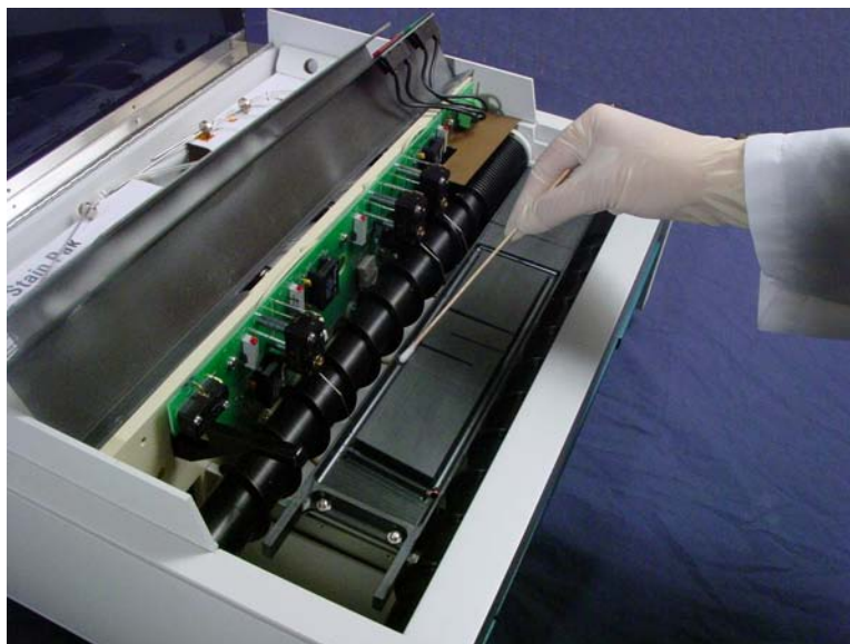
Figure 5-6. Cleaning the Back Trough
