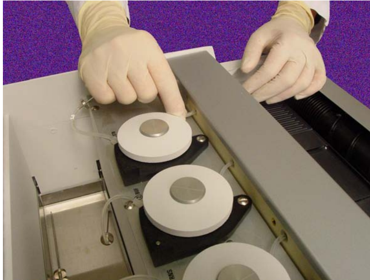
Figure 2-4. Attaching Pump Tubing to Nipple
