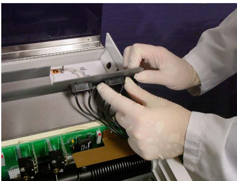
Figure 6-6. Unsnapping the Light Assembly
