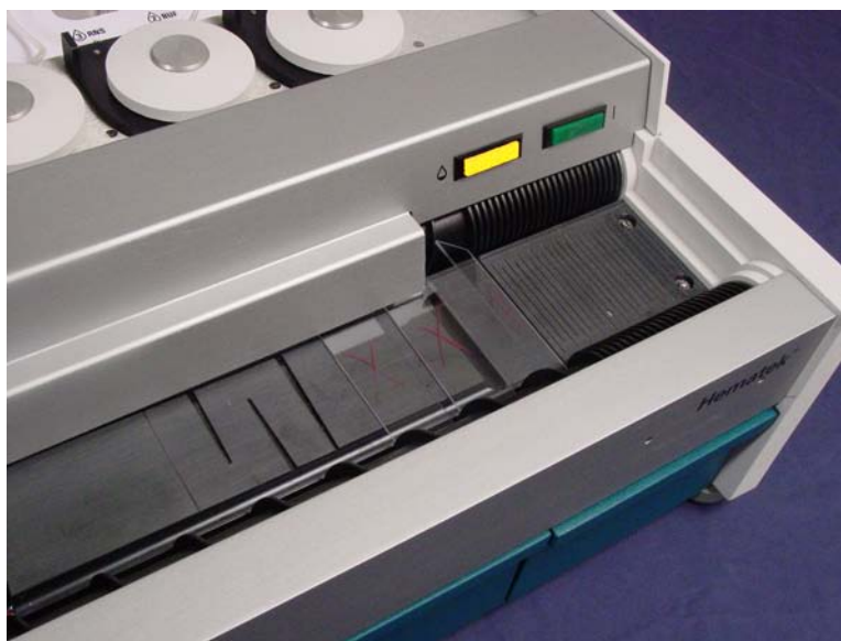
Figure 3-2. Priming the Platen
