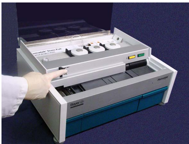
Figure 6-7. Priming the Tubing
