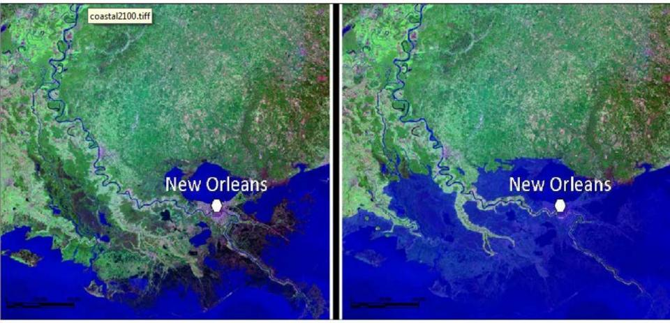
Map: Blum, M.D., and H.H. Roberts (2009), Drowning of the Mississippi delta due to insufficient sediment supply and global sea-level rise, *Nat. Geosci.*, 2, 488-491. Using the GPS Surveying Equipment and the C4G Real Time Network, we know LA 1 lost over 1 foot of elevation in just 20 years.
