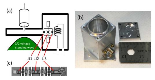
**Fig. 1.** The Zappe photon upconverter. (a) A schematic of the 3D microwave cavity and the Zappe interferometer coupling to the Compton frequency signal flowing through the inductor. The 3 Josephson junctions in the Zappe interferometer are labeled JJ1, JJ2, and JJ3. (b) A photograph of a prototype microwave cavity. (c) A prototype of the Zappe interferometer, with the 3 JJs labeled.
