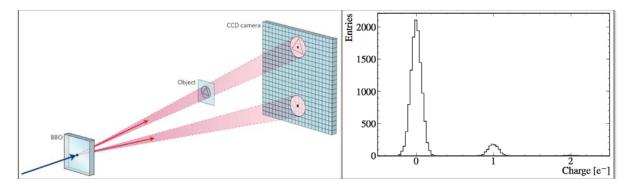
Figure 1. Left) The differential quantum imaging experiment. The  $\beta$ -barium borate (BBO) crystal produced an entangled pair which is then imaged with a CCD camera. Non-classical correlations are used for the improved differential imaging of a weakly absorbing object. [Figure from Nature Photonics] Right) Photon counting capabilities of the skipper-CCD, showing the signal for zero and 1 photo-electrons.
