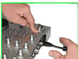
If neither occur, unplug the device and try again, making sure to press and hold the **Mic On/Off** button before plugging in the device, and maintaining the hold thereafter
