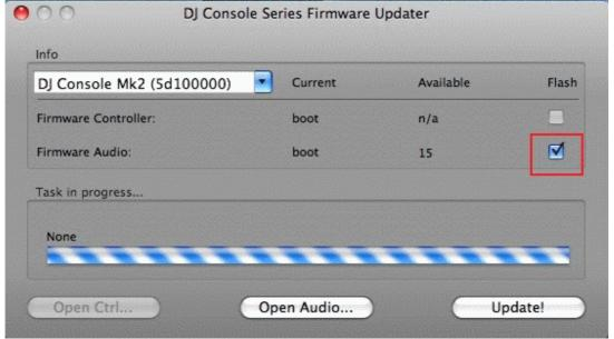
THE CONSOLE MUST NOT BE UNPLUGGED until the manual updater confirms completion and advises to do so
