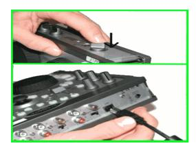
b) If the *Current* column does not show boot OR the device is still not detected, unplug and re-plug again following the same procedure, making sure to press and hold the TALK-Over button before plugging in the device, and still maintaining the hold once connected
