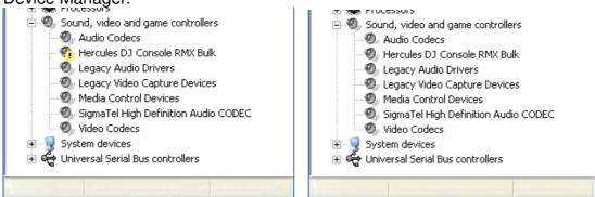
Whether or not the bulk device (*Hercules DJ Console RMX Bulk*) is enumerated correctly, right-click on it and select **Uninstall**.
