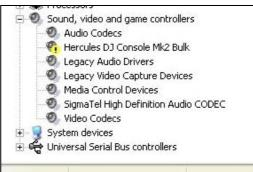
Whether or not the bulk device (*Hercules DJ Console MK2 Bulk*) is enumerated correctly, right-click on it and select **Uninstall**.
