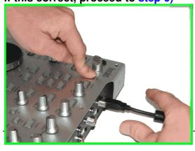
b) If the *Current* column does not show boot OR the device is still not detected, unplug and re-plug again following the same procedure, making sure to press and hold the MIC On/Off button before plugging in the device, and still maintaining the hold once connected
