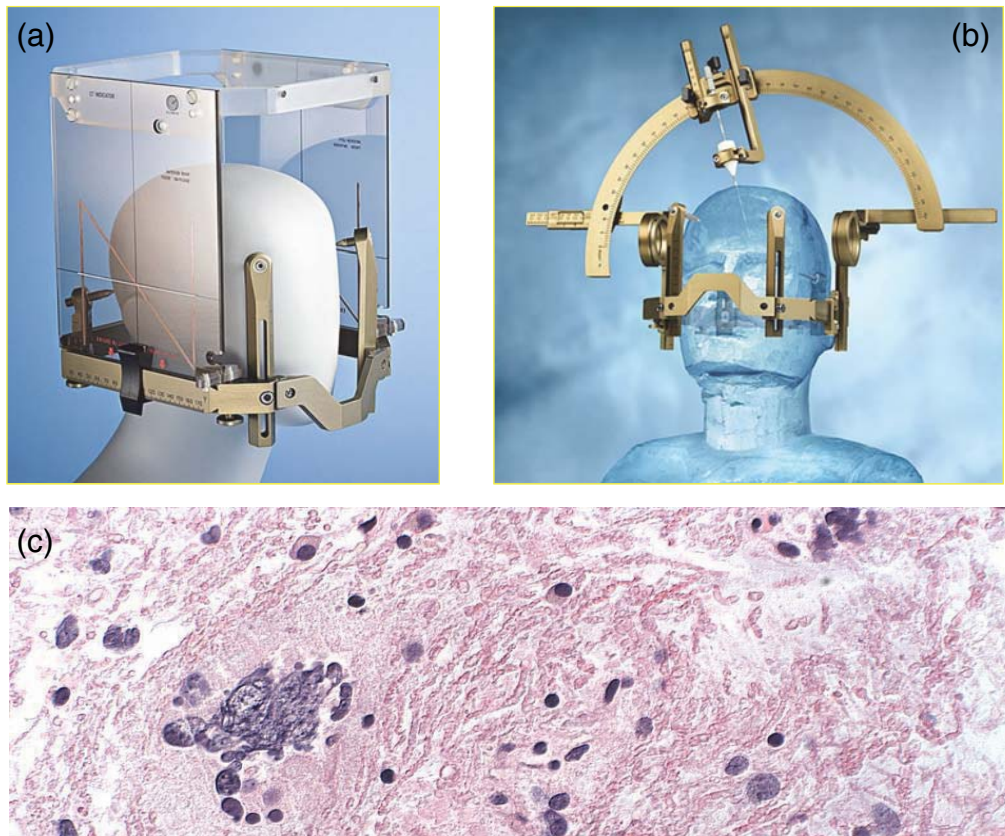
Figure 1.9 A stereotactic fine-needle biopsy device consists of an immobile frame screwed firmly into the skull in the operating room, along with two separate attachments used in sequence. (a) The first of these consists of an array of paramagnetic fiducial markers embedded in plastic planes; these can be read precisely by the MRI device during a clinical study. These make possible accurate localization of a target point within the lesion. (b) Then, with the frame still fastened rigidly to the skull, the first assembly is removed and a second attached. This one can guide insertion of a hollow sampling needle along any direction chosen by the neurosurgeon, such that its tip will end up within 1 mm of the target point. [Courtesy of Elekta]. (c) Photomicrograph from one of the biopsy slides. The pathologist reported that the sample collected from this lesion displays scattered and atypical cellular nuclei, suggestive of an astrocytoma, a form of glioma, but of undeterminable grade.
