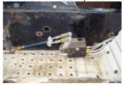
Here is my mechanical brake bias. The mechanical bias is attached to the pedal with all thread rod. I used some blue fuel line and slid it over the rod to give it a better look.
