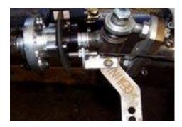
Here is an up close look at the mounting I make for the mph sensor which connects to my Digatron Tach. It is a magnetic type switch and trips everytime one of the dowels the rotor floats on passes by them.
