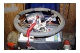
Here is the throttle setup ast the carbs. I use a throttle linkage kit from E.C. I believe the part number is lk-122. I do modify it just a bit, but each application will be different.
