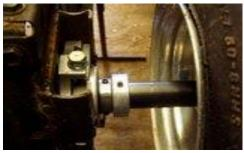
Here you can see the lock collars. E.C. sells these, and I use them outside each axle bearing like in the pic to keep axle in place, both sides of wheel hubs and both sides of brake and sprocket hubs. In this build case the brake hub is against the bearing hub so it only required one side. A total of 9 on this setup where I usually use 10.
