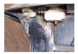
On MTD's without side panels, to hold the grill, they have two rods that attach to the dash. I weld a 1/4" thick flat bar to the dash support cage so it has something to bolt to besides the plastic dash.
