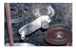
Here is the pitman arm on the end of the shaft. The next photo will show you the depth from where it comes thru the frame to the bottom of the frame.
