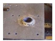
Here it is welded completely in place. This bushing supports the weakest link (the input shaft) of the 700 tranny and with this setup if you break the input shaft it is due to case fatigue or worn or bad bearings.
