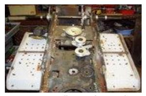
Here is an overall view of rear axle in place, with tranny pulley and clutch and guides in place. Also, notice the center of the running board rod is cut out as described in earlier details. This gives wide open access to everything.
