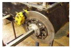
Here is an overall view of the brakes and rotor. Yup its a big rotor but the bigger it is the less force needed to stop it. It is a motorcycle rotor redrilled to fit the MCP brake hub. Everything is setup so the rotor hub is against the bearing hub and I put a slit collar outside the brake hub to hold it all in place. The caliper is bolted to the
