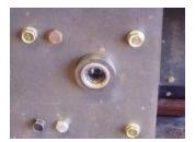
As you can see it aligns perfectly. Now tack it in place and then remove the tranny case wnd weld it completely in.
