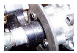
Here you see the rotor and the pins/dowels it floats on. When shimming between hub and caliper, be sure you do not shim so much. The rotor will float off the pins. This could result in a nasty ride at the end of the straight.
