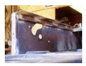
Now this is inside the side frame panels. I use the same tubing to stiffen the box or tunnel of the frame. Makes for a solid chassis and it isn't add much extra weight either.
