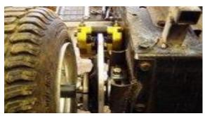
Here you can see the clearance between caliper and tire. Tire 19 inches from center of frame. That's the outer sidewall.
