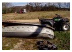
This is a handy tool an aluminum yard stick. Being very flexible makes it a good straight edge, even on rounded surface. I clamp it on one end, then hold it on the other and mark it with a sharpie. Then cut the bottom off.
