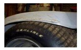
With my tallest tire on the mower (turf Masters), you see they fit and still have right at a 1/4 inch clearance. The chassis is 4-1/8 inch off the ground on the rear. And nothing has been cut.
