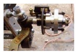
Above is a close up of the Hegar front brakes. The axle is keyed with a 3/16 key and has 2 set screws to keep it tight. Never had any trouble with these brakes.
