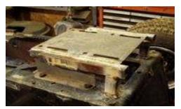
Here is a better view of what I have done. You can see at the rear where I added an upright support with same size tubing. Fender will bolt down on top of all this and seat will bolt into the slotted grooves where it gives you the ability to slide the seat forward or backwards the original amount. ALL legal and great for fine tuning the handling of your mower. Fenders will still bolt into the original holes in the running boards giving the appearance they haven't been moved.
