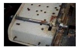
Here is the brake pedal, I used an arm from an extra steering kit I had for the linkage mount. I slotted the running board so it sticks up thru it on the top side. Notice I don't have the center mount on this pedal. It doesn't receive all the vibration the clutch pedal gets from the belt. So it isn't needed.
