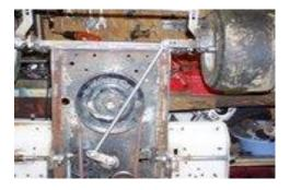
Here is an overall view of my steering set up with the E.C. Axle. I have been using this setup for going on 5 years now. I love it. ¼, maybe a tad more, is all you will ever turn the wheel in a race.
