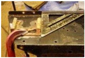
You want to make sure that both sides are the same in the case of this chassis I measured from the front of the frame side panel to the front edge of the cassette holder, (28-7/8) and from the top of the side panel to the top of the holder (2-1/4) and be sure you have it square to the frame. All these measurements are decided using the shortest tire I run. And if using adjustable cassettes you will generally have as much as 3/8 up and down adjustability in your ride height.
