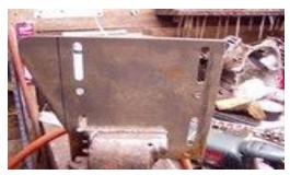
Now on the top side of the chassis with the axle and wheels on I turn to working on fender mount and seat mount for wheel clearance. Anyone taking a mtd apart or knows them, knows the full fenders are mounted on a channel type pedestal. I reuse these. I cut the factory seat bracket the inside width of these pedestals.
