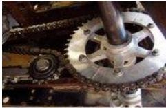
Here is a closer look at the idler adjuster that we make and sell at EC to go with the tranny plate. It and the Idler sprocket is sold separately. It has 4 holes in tranny plate to make adjusting, no matter what the slack in chain is, relatively easy.
