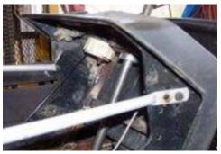
Here are the grill support rods bolted to the dash.and the bar I weld in. I drill and tap for 1/4 threads, then simply run a bolt in, no nut. Makes for quick removal.
