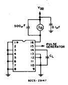
Fig. 10 - Power-dissipation test circuit.
