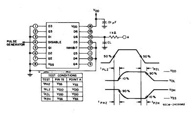
Fig. 14 — Disable delay times test circuit and waveforms.
