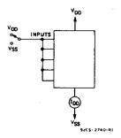
Fig. 11 — Quiescent-device-current test circuit.
