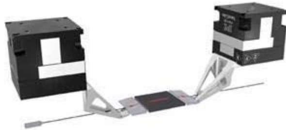
Figure 3. PI Probe Station Concept for Individual PICs.
