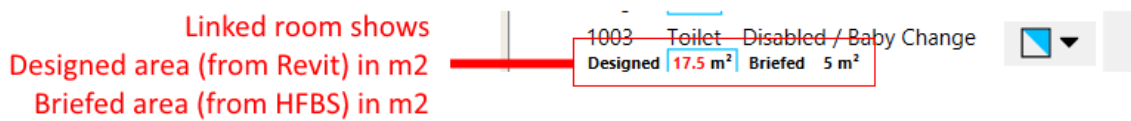
Figure 37 Project Manager window - Designed area from Revit, vs Briefed area from HFBS is displayed under rooms and departments.
