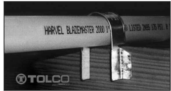
Tolco Hanger/Restraiter can function as a hanger or as a restrainer and can be mounted from the top or bottom of a beam. The fastener mounting edges are designed to allow the screws to be installed horizontally. This is a benefit when overhead clearance is limited.
