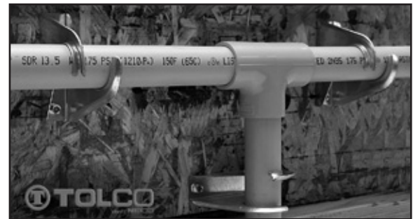
Tolco Stand-Off Hanger/Restraiter can function as a hanger or as a restrainer for installations where a standard offset is required. The Stand-Off Hanger can perform as both a hanger and restrainer on horizontal piping, and as a stabilizer for vertical sprinkler head drops. The manufacturer furnishes listed fasteners for use into wood.
