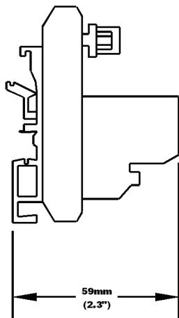
**FIG. 3-11 RTA DIN RAIL MOUNT**
