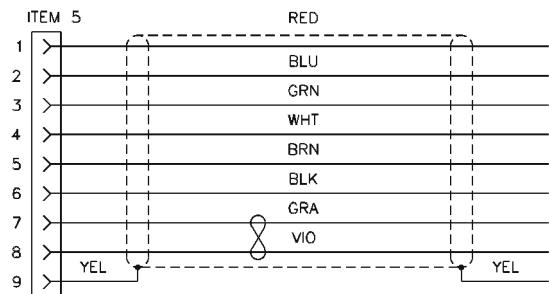
**FIG. 3-13 RTA CABLE SCHEMATIC - HI 1769-WS**
