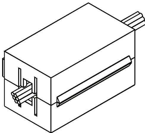
**FIG. 3-18 SUPPRESSION CORE INSTALLED**
