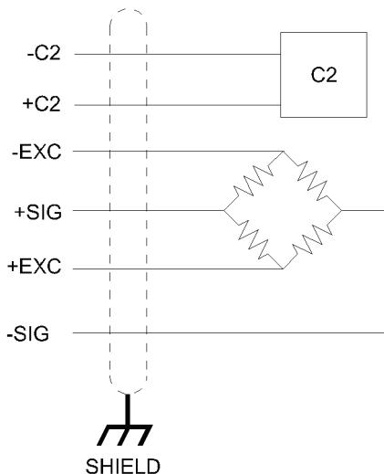
**FIG. 3-9 HARDY LOAD SENSOR/C2 WIRING
