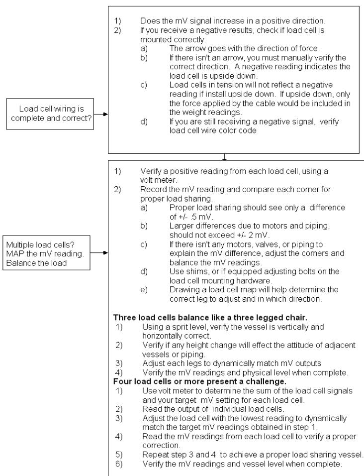
**FIG. 6-2 LOAD SHARING AND LOAD SENSOR CHECKOUT**
