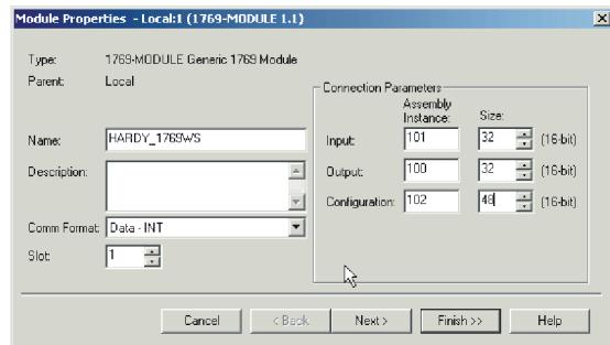
**FIG. 4-12 MODULE PROPERTIES DIALOG BOX/CONFIGURATION/SIZE/48 WORDS**
