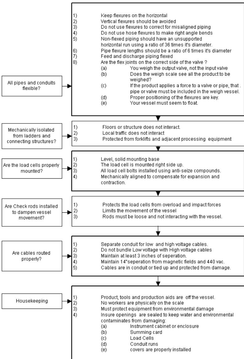
**FIG. 6-1 MECHANICAL INSPECTION**
