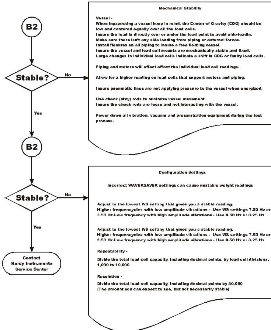
**FIG. 6-5 MECHANICAL STABILITY AND CONFIGURATION SETTINGS**
