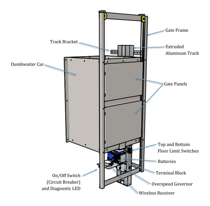
The dumbwaiter car is fully assembled onto the chassis and bottom piece of track. If necessary, the car can be removed from the chassis for installation.
