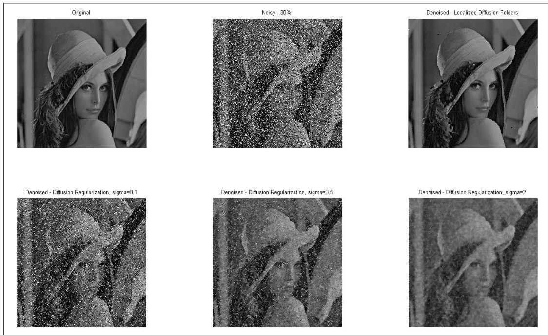
Figure 4.6: Comparison between the denoising results of the LDF and the diffusion regularization algorithms
