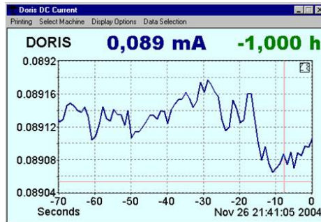
Figure 4: Beam current versus time measured in DORIS over one minute.
