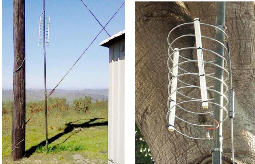
Figure 2: (A) at club's remote base site. (B) Hiding in the big oak tree behind my house. Note balun and turn-shortening jumper.
