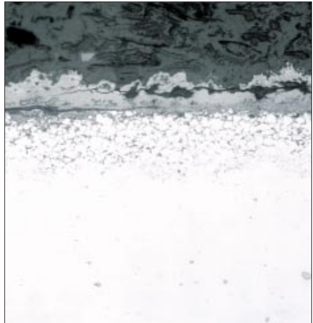
Figure 53 - Intergranular oxidation. (200X)
