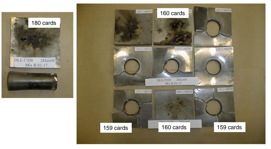
DLE-C038 card gap of 160 cards compares well to the PBXN-110 card gap of 156-178 cards
