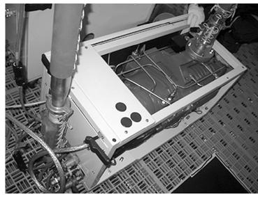
The use of rotary vane vacuum pumps to support a number of different types of process equipment is widespread in industry. Semiconductor cleanroom facilities, laboratories, pharmaceutical, and biotech facilities rely heavily on the use of vacuum pumps. Vacuum pumps typically account for 5-20% of a semiconductor
