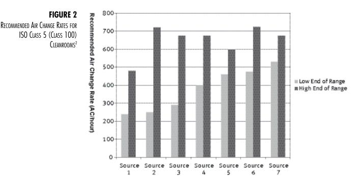
Using better air change rate practices will allow designers to lower construction costs as well as reduced energy costs while maintaining the high level of air cleanliness that is required in cleanroom facilities.
