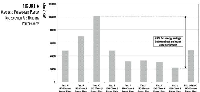
The figure above shows the variation in performance between pressurized plenum recirculation air systems as found in the LBNL Benchmarking project. The worst performer was the cleanroom in Facility J at 2185 cfm/kW. The best performer was the cleanroom in Facility C. The best performer saved 78% of the fan energy of the worst performer.
