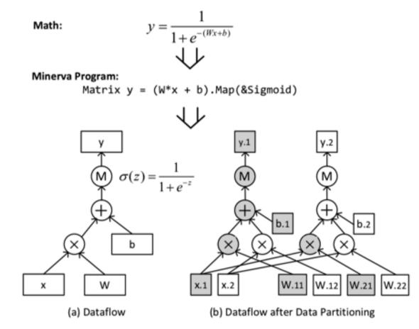
Statement and its dataflow fragment. The data and computing vertexes with different colors reside on different processes.
