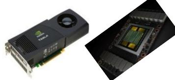
Accelerators high compute density, high performance/watt >1 TFlop DP on a chip
