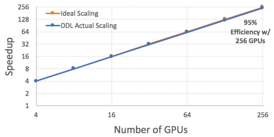
Caffe with PowerAI DDL on ResNet-50 model using the ImageNet-1K data set on 64 Power8 servers
