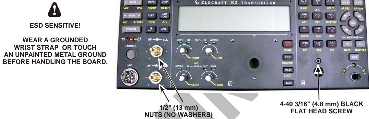
Figure 37. Mounting the Front Panel on the Front Panel Board.
