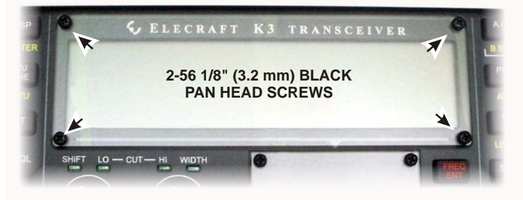
Figure 41. Installing LCD Cover.
