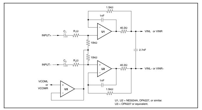
Figure 51. Alternative Buffer Circuit Using Standard Op Amps
