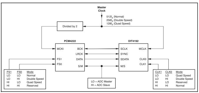
Figure 53. Interfacing the PCM4222 to a DIT4192
