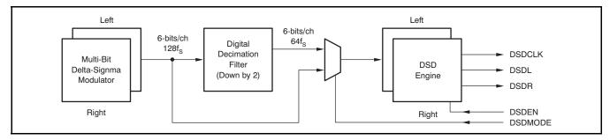
Figure 46. Simplified Block Diagram for DSD Mode Operation
