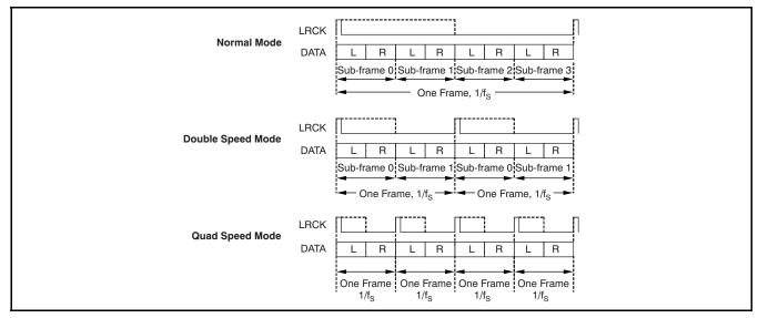
Each L or R channel time slot is 32-bits long, with 24-bit data Left-Justified in the time slot. Audio data is MSB first. Sub-frame assignments for each PCM4222 device are selected by the corresponding SUB0 and SUB1 pin settings.
