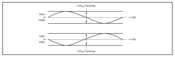
Figure 37. Full-Scale Analog Input Range
