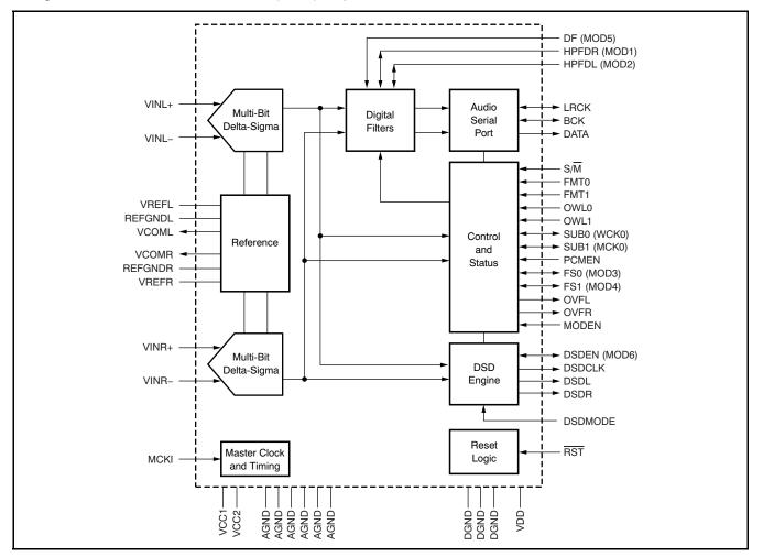
Figure 36. Functional Block Diagram
