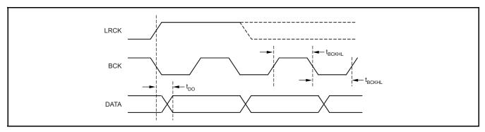
Figure 2. Audio Serial Port Timing: TDM Data Formats
