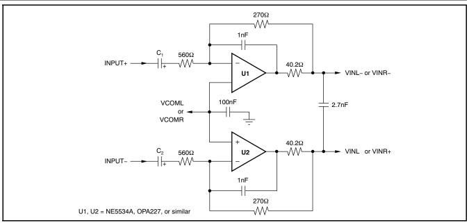
C1 and C2 provide ac coupling. They may be removed if the dc offset from the preceeding circuit is negligible.
