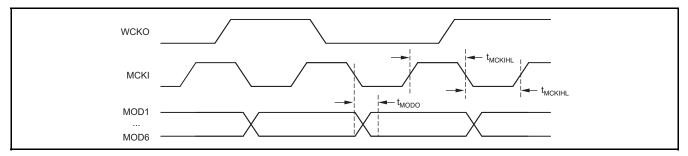
Figure 4. Multi-Bit Modulator (MBM) Output Timing
