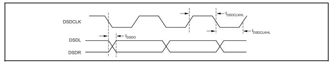
Figure 3. Direct Stream Digital (DSD) Output Timing
