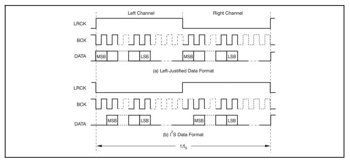
Figure 42. Left-Justified and I<sup>2</sup>S Data Formats
