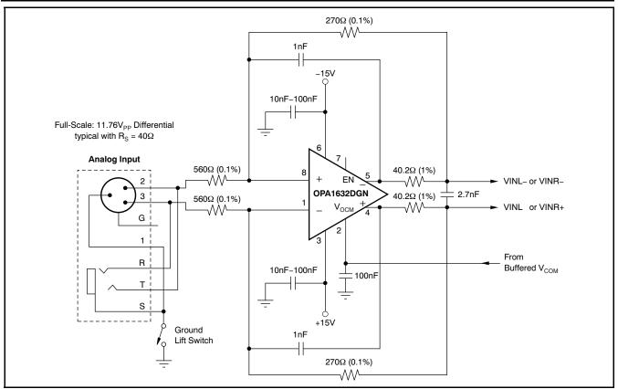
Figure 50. Differential Input Buffer Circuit Utilizing the OPA1632
