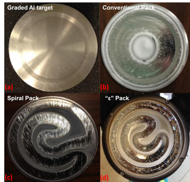
Fig. 10. (Color online) (a) Graded 4 in. Al target. (b) Race track erosion pattern on the 4 in. Al target from conventional magnet pack. (c) Race track erosion pattern on the 4 in. Al target from spiral magnet pack. (d) Race track erosion pattern on the 4 in. Al target from \epsilon pack.
