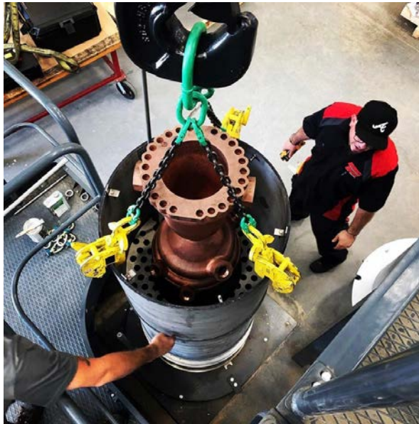
Figure 3. Additively manufactured rocket engine thermally processed using HIP and heat treatment in the same cycle – High Pressure Heat Treatment
