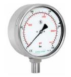
BOTTOM CONNECTION Range of WP available: Up to 6000 bar Connections available: 1/2" BSP, 1/2" NPT, 9/16"-18 UNF Units: Bar/psi
