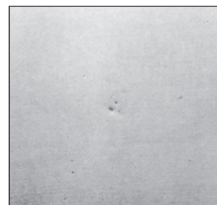
Pinhole texture by inappropriate rust proof.
