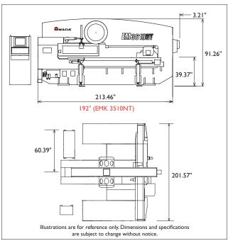
The dimensions for the EMK 3510NT and the EMK 3610NT are identical except for overall length (indicated in red).
