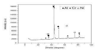
Figure 7: XRD pattern of Ni<sub>22</sub>Cr<sub>11</sub>Al powders sintered at 1100°C.
