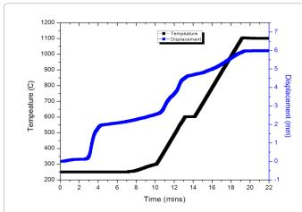
Figure 3c: temperature and displacement curve in spark plasma sintering process at 1100°C.
