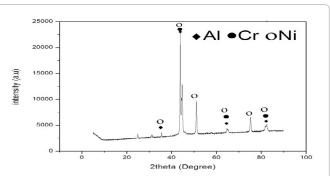
Figure 6: XRD Pattern of  $Ni_{22}Cr_{11}Al$  powders sintered at 1050°C.
