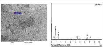
Figure 5: SEM micrograph of Ni<sub>22</sub>Cr<sub>11</sub>Al powder (Left), EDS analysis (Right) sintered at 1100°C.
