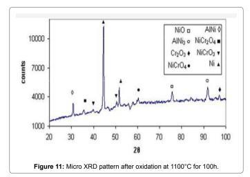
of the TGO reveals the high percentage of  $O_2$  and Al and less of Cr and Ni element. Hence the main component of the TGO is  $Al_2O_3$
