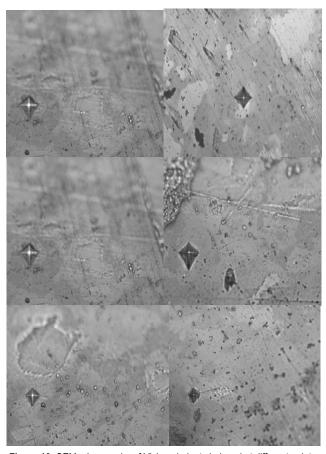
Figure 10: SEM micrographs of Vickers indents induced at different points.
