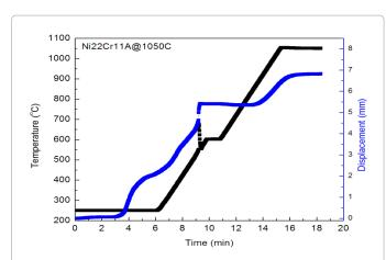
Figure 3b: The temperature and displacement curve in spark plasma sintering process at 1050°C.
