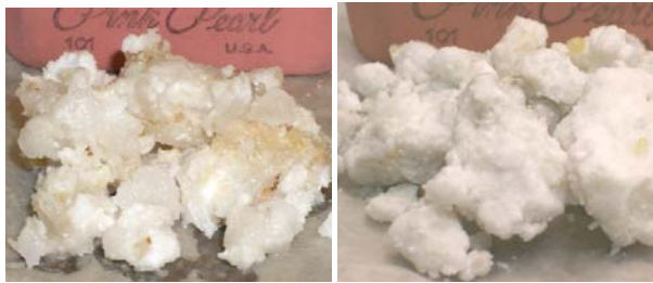
3 a. 3 b. Figure 3: Calcium silicate hydrate (a) 16 hours at 250 °C, P_{H_2O} = \sim 680\text{PSI} (b) 7 days at 250 °C, P_{H_2O} = \sim 680\text{PSI}
