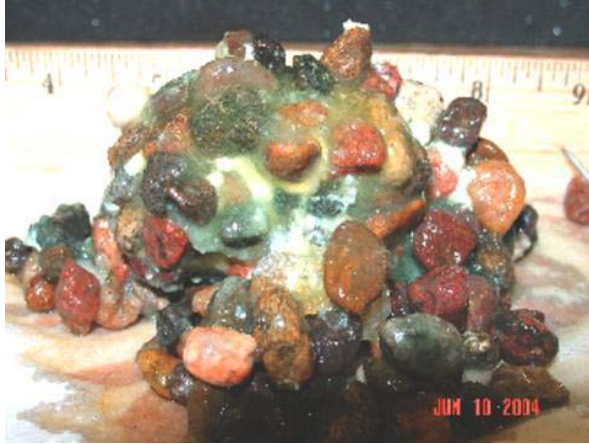
Figure 4. Gravel and calcium silicate hydrate agglomerate formed at 90°C.
