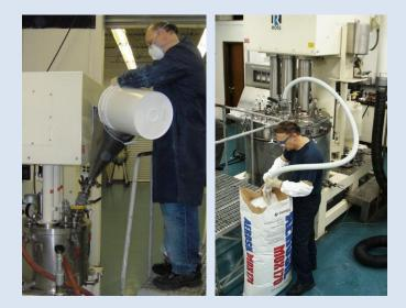
Mixers operating with multiple agitators are exceptionally versatile, but they still have limitations in their range of viscosity. Their versatility mainly results from independently-controlled drives: the agitators can be engaged in any combination and at any speed for any interval during the mixing cycle. Although this sounds complex, multi-shaft mixers are actually engineered to be comparatively simple, effective and economical.
