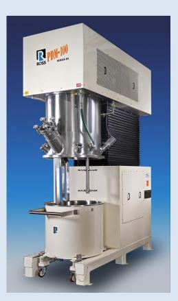
Powders consisting of talc, kaolin clay, silica, graphite, etc. are loaded into the PowerMix, followed by the liquid component. The combination of high speed mixing and planetary stirring produces the same dispersion quality as the control sample in less than half the time it takes in the double planetary mixer. In under 40 minutes, a better quality slurry is completed in the 40gallon PowerMix with a final viscosity of ~120,000 cP.
