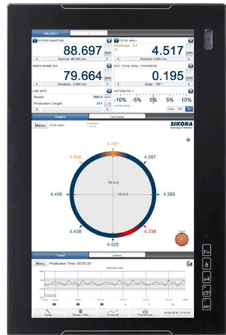
The production data of the X-RAY 6000 PRO is clearly displayed on the vertical 22" wide-screen monitor ECOCONTROL 6000
