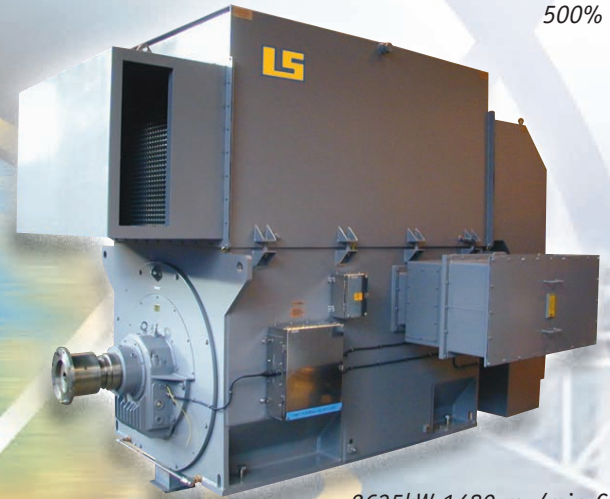
2635kW 1480 rev/min CACA 6600V 3ph 50Hz Water Injection Pump Motor 300% FLC
