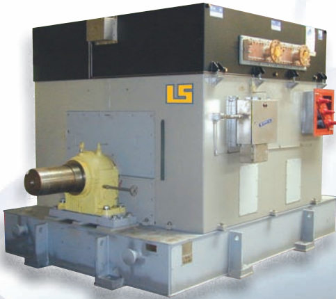
10750kW 1770 rev/min CACW 13800V 3ph 60Hz LP/IP Compressor Drive Motor 320% FLC
