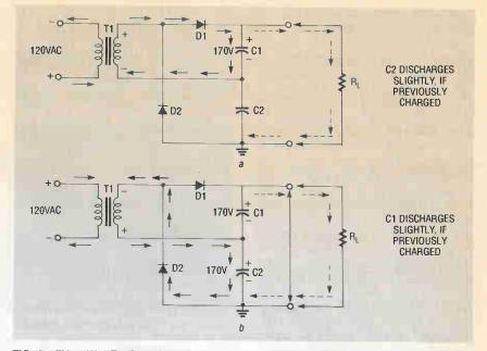
FIG. 3—FULL-WAVE VOLTAGE DOUBLER, redrawn for greater clarity. For the first halfcycle (*a*), D2 is cut off and D1 conducts, producing about 170 volts DC across C1. On the next half-cycle (*b*), D2 conducts and D1 is cut off. The output voltage is now across C1 and C2 in series, doubling the level to about 340 volts DC.
