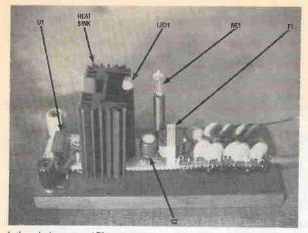
In the author's prototype, LEDI and NEI were mounted to 1/2-inch stand-offs, and the entire circuit (minus the power supply) was mounted to a block of wood. The wood block helps to isolate and insulate the circuit board from any metallic objects.
