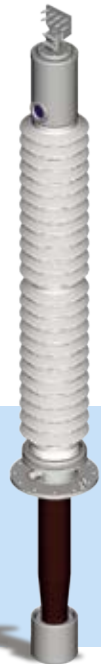
"Air-oil" bushings for power transformers and shunt reactors Voltage: 12–1200 kV Current: 315–2500 A
