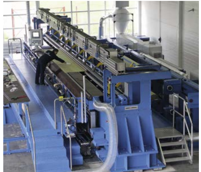
Manufacturing of bushing main insulation in Izolyator factory
