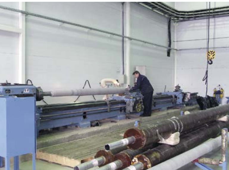
Fig. 10. Lathe turning of 252 kV RIP-insulation at the Izolyator plant
