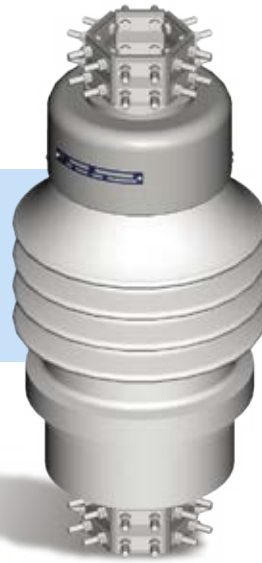
"Air-oil" bushings for oil switches Voltage: 40.5–252 kV Current: 1000–3150 A
