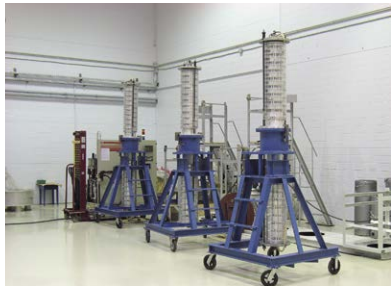
Fig. 13. Direct molding of silicon rubber on solid RIP-insulation at the Izolyator plant
