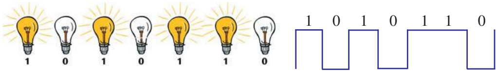
Fig. 1.8 : Digital representation of ON and OFF states
