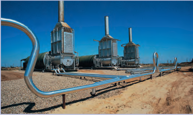
Figure 3: Pipeline for oil transport from the separators nearly situated at the wells to further processing
