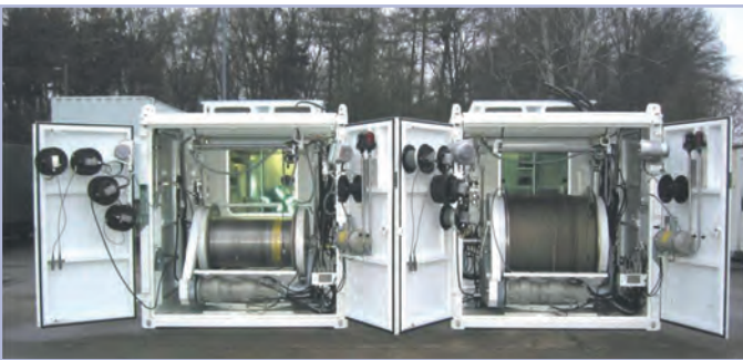
Figure 7: A winch in a container for offshore applications.
