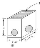
Used when height of inlet is 6' - 0" or less.
