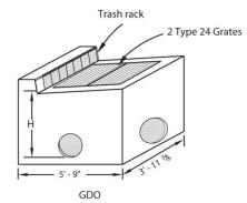
Trash rack provided when needed. Use with Types A and B curbs and Type A dike, or recessed in a cut slope.
