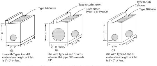
NOTES: 1. All dimensions are outside dimensions based on 6" wall thickness.
