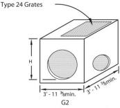
Use with Types A, B, and D dikes when outlet pipe O.D. exceeds 24".
