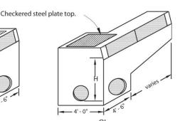
OL Curb opening lengths 7', 10', 14' and 21'. Use only with Type A and B curbs.
