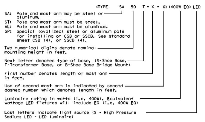
Figure 5-1. Explanation of roadway illumination assembly codes.
