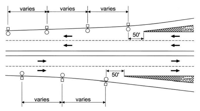
*Figure 6-2. Typical placement for partial interchange lighting, 40 foot luminaire poles at merge and diverge lanes.*
