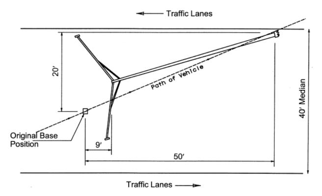
Figure 6-3. Falling area - final position of 50 foot luminaire support.
