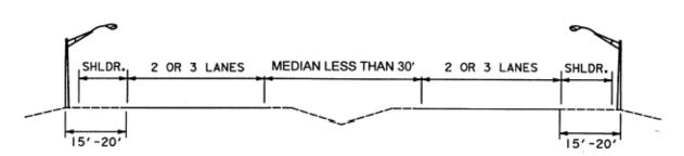
Figure 6-4. Typical house-side lighting for controlled access highway. In this example: Luminaires are 250W EQ LED - Mounting Height is 40 feet. - Spacing varies (see Section 6 of this chapter, Spacing of Light Poles).
