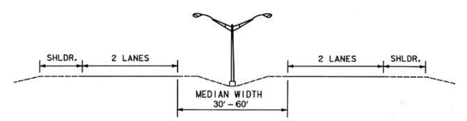
Figure 6-5. Median lighting with breakaway poles.
