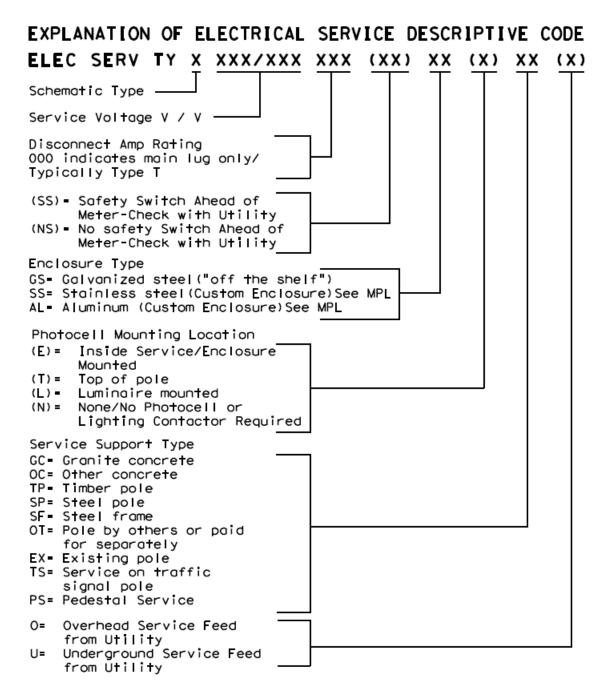
*Figure 5-3. Explanation of electrical service descriptive code.*
