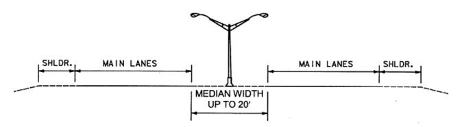
Figure 6-6. Median lighting with concrete median barrier.
