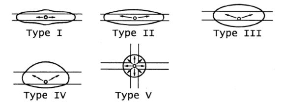
Figure 5-2. Plan views of light distribution patterns for basic types of conventional luminaires.
