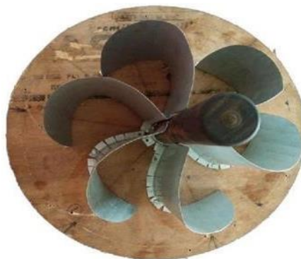
Fig: Turbine with six number of Blades
