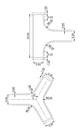
Minimum turning head Dimensions for 5.5m Carriageway.
