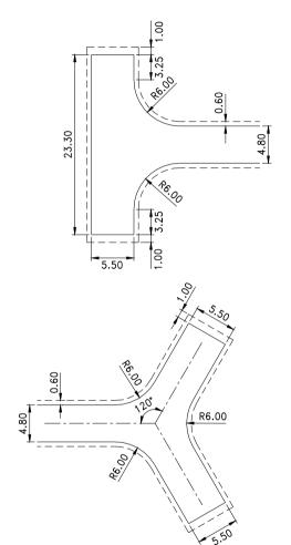
Minimum turning head Dimensions for 4.8m Carriageway.
