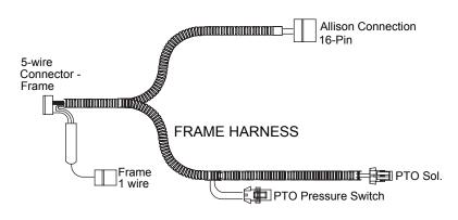
Locate the wiring harnesses provided in this kit. The harness can be separated into two sections. The section without the loom is for inside the cab. Pull the fuse
