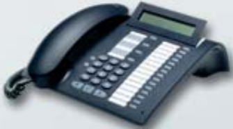
optiPoint 500 advance The telephone for professionals with: • illuminated display • 2 adapter ports • 19 function keys with LED • integrated interface for headset
